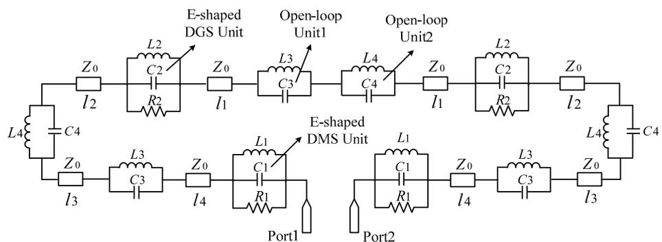
**Fig. 2.** Equivalent circuit model of the proposed filter.
