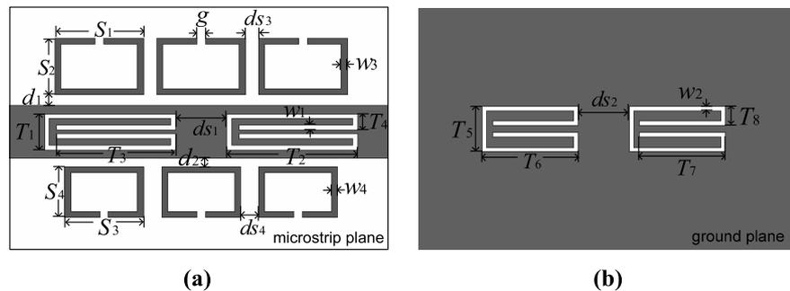
**Fig. 1.** Configuration of the proposed quad-band bandstop filter. (a) Top microstrip plane. (b) Bottom ground plane.
