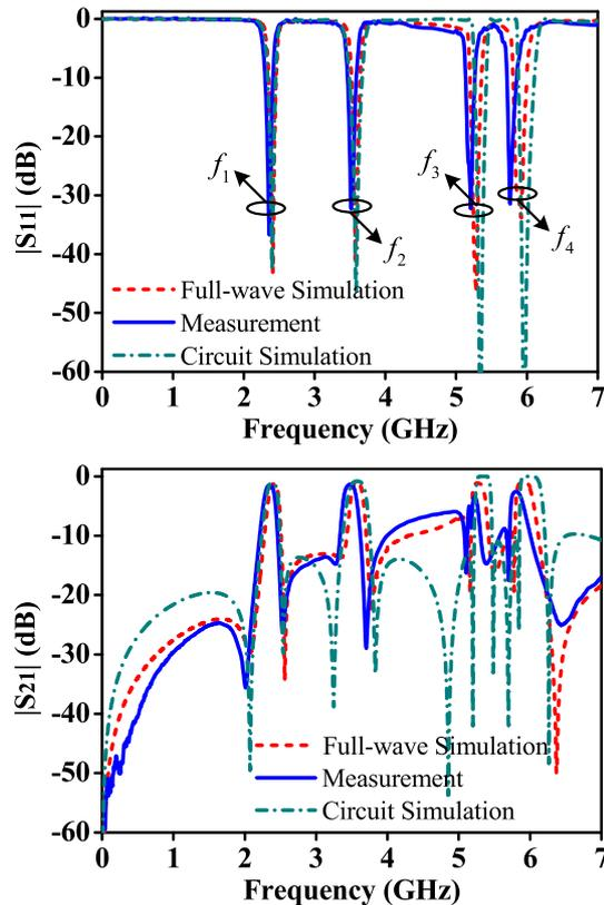
Fig. 4. Simulated and measured S-parameters of the fabricated filter.
