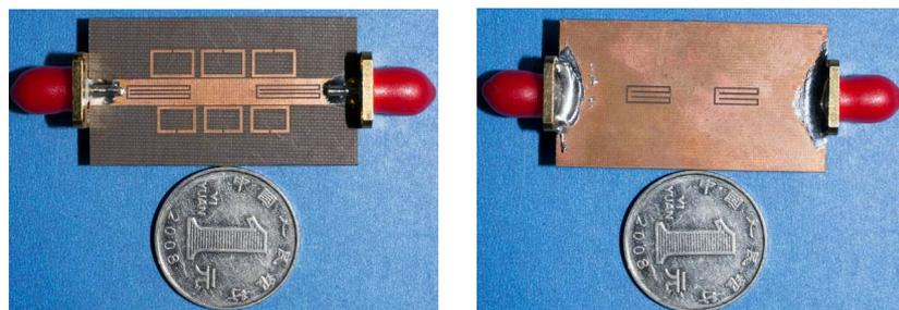
**Fig. 3.** Photograph of the fabricated quad-band bandstop filter.
